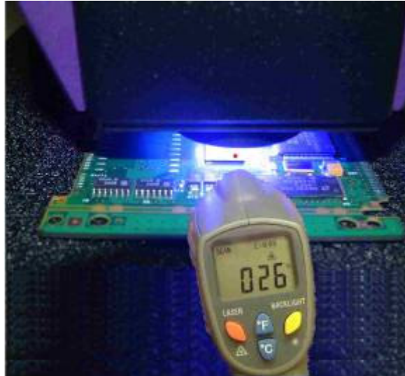
Figure 6. Heat sensitive media are an ideal fit with SLM light sources, which only heat the media slightly above ambient temperatures during the cure cycle.
