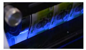
UV inks don't require the attention when ink colors are changed, and different media can be run on the same press without the need for time-consuming cleaning of equipment, greatly reducing downtime. Operators can run the machines day in and day out without having to stop, which increases the amount of time the presses are running to 90 percent, a substantial uptime gain with a proportional rise in operational savings.
