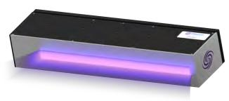
The beauty of LEDs is that they instantly turn on or off. As a result, the UV source is cycled on/off as needed and interlocked to material-handling equipment so that if any production stops occur, the light immediately switches off and then back on as soon as the line starts again.
