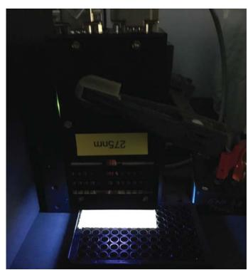
The air-cooled 275 nm UV LED lamp shown here (as used in these experiments) was constructed with continuous adjustable power control allowing control of the dose delivered at target in specific time frames. The lamp has an emitting window size of 75x20mm and, in this photograph, was positioned 10 mm from the glass slide target surface.
