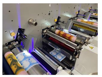
LED curing was successfully installed and put into operation. The machine consumes approximately 60% less electricity, which corresponds to an annual saving of approximately 84,000 kWh, eliminating 200 tons of CO<sub>2</sub>.
