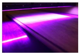
UV LED curing offers lower operating costs, enhanced system capabilities due to being a solid-state device, and significant environmental benefits. Traditional mercury UV lamps generate a tremendous amount of heat, requiring both a significant amount of electricity and cumbersome air-handling infrastructure to operate. By replacing the mercury UV lamps with UV LED curing systems, customers have experienced energy savings of up to 85 percent.
