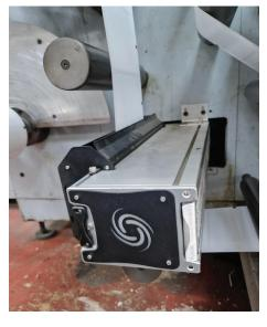
Reel Appeal decided to retrofit one of their Rhyguan finishing machines with the Phoseon Nexus ONE™ 375 aircooled UV LED curing system to improve their offerings for customers. Upgrading their machine from UV to Phoseon Nexus ONE enables them to print and varnish using LED technology.
